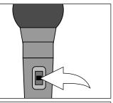
To turn the microphone on, slide the ON/OFF switch, located on the side of the microphone, to the ON position. To turn the microphone off, slide the ON/OFF switch to the OFF position.
